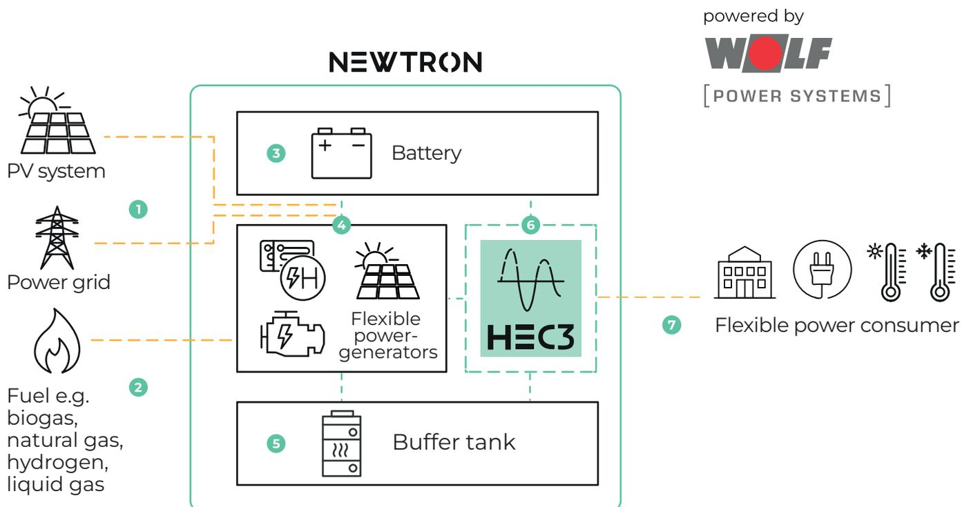
HEC3 is the managing core and possess the standardized interface to different energy components, which are configured as requested. With the HEC3 energy management system, energy flows are identified and flexibilities are actively traded on the electricity market.
