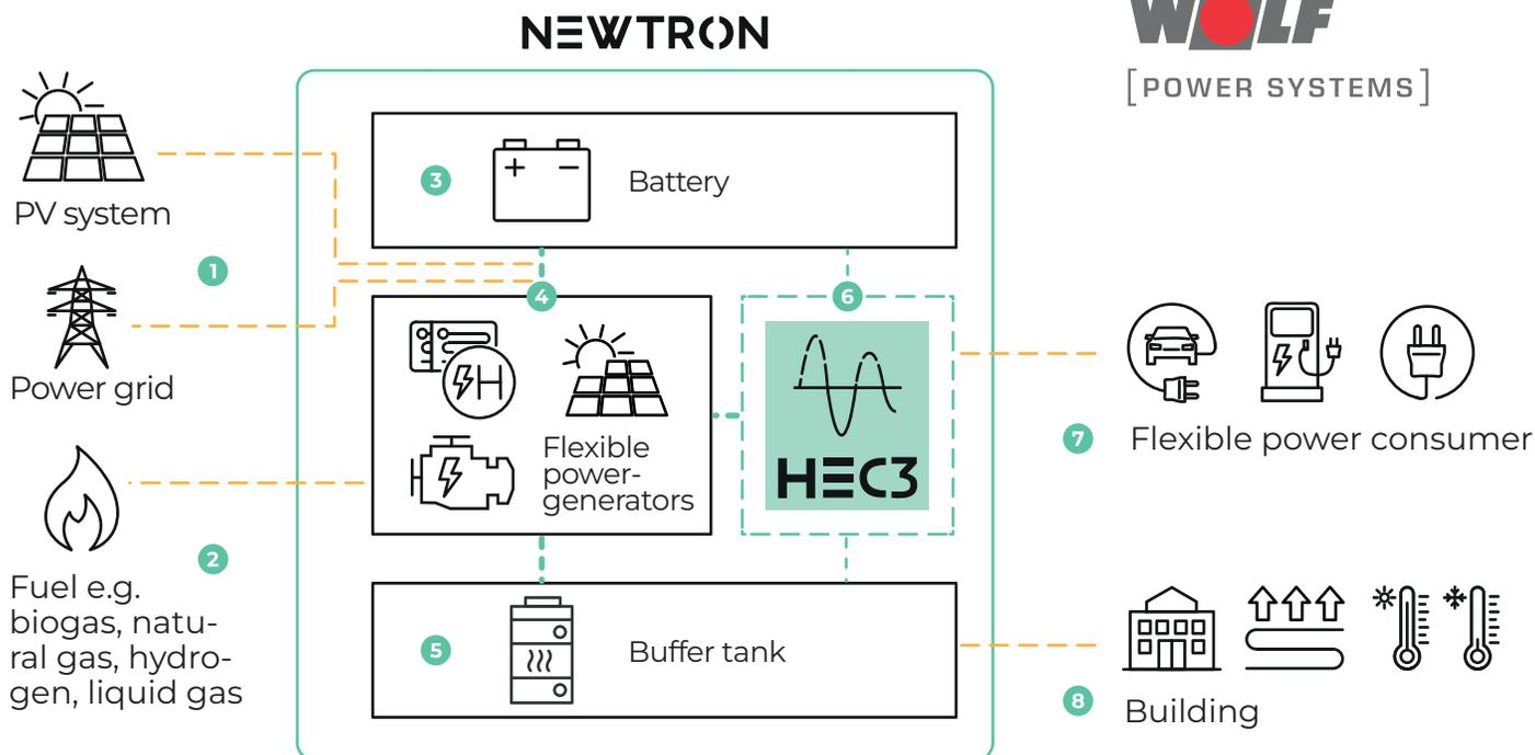
HEC3 is the managing core and possess the standardized interface to different energy components, which are configured as requested. With the HEC3 energy management system, energy flows are identified and flexibilities are actively traded on the electricity market.
